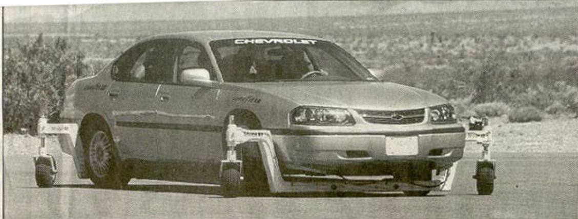
On the skid-control course, drivers use an Impala with a hydraulic frame that the instructor can manipulate to reduce front or rear traction to show what causes a skid and how it can be controlled.
